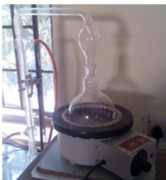
**Fig. 13.** Distillation unit
