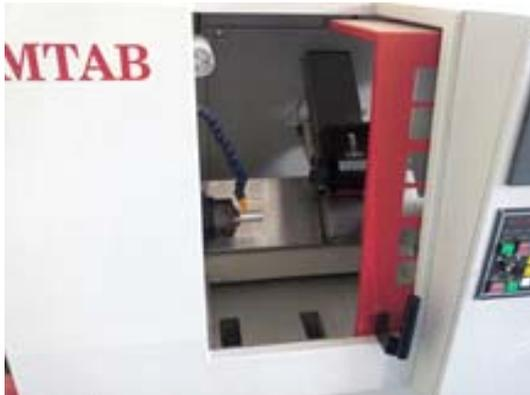
Fig. 1. Application of cutting fluid during an experiment
