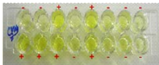
Fig. 2. Detection of CMV from symptomatic gherkin plants through DAS-ELISA. Yellow colour - positive; No colour development – negative
