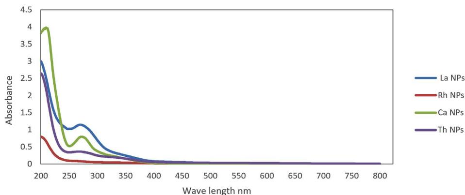
**Fig. 3.** UV-Vis absorbance of La, Rh, Ca and Th silver nanoparticles.
