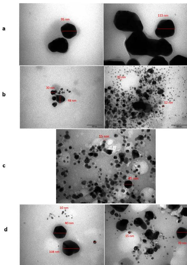
**Fig 4.** TEM images of a) La, b)Rh, c) Ca and d) Th silver nanoparticles.
